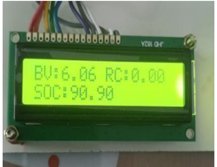
Fig 9.4 90% Battery in Approximately 130 Min
